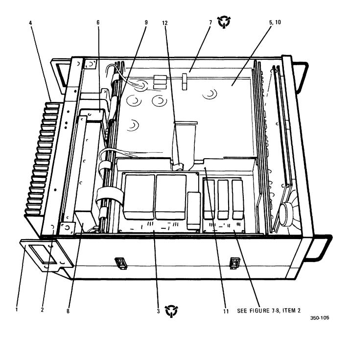
Figure 7-5. 100 Watt Transceiver, RT-1446/URC, Top Side View
