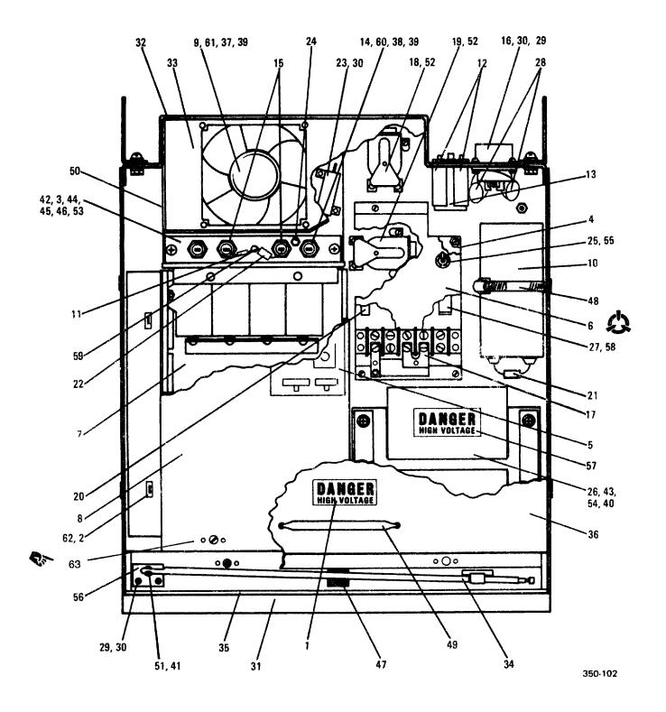
Figure 7-2.100 Watt Transceiver, RT-1446/URC, Bottom Half
