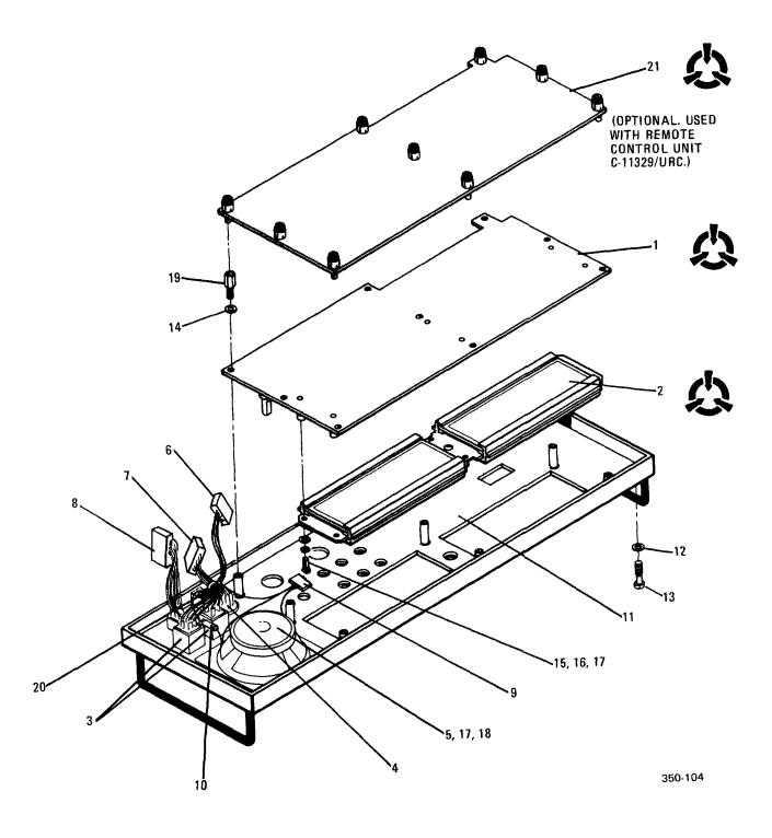
Figure 7-4. 100 Watt Transceiver, RT-1446/URC, Front Panel Assy, A1A11
