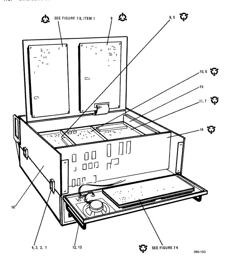
Figure 7-3. 100 Watt Transceiver, RT-1446/URC, Internal Components (7-19 Blank)/7-20
